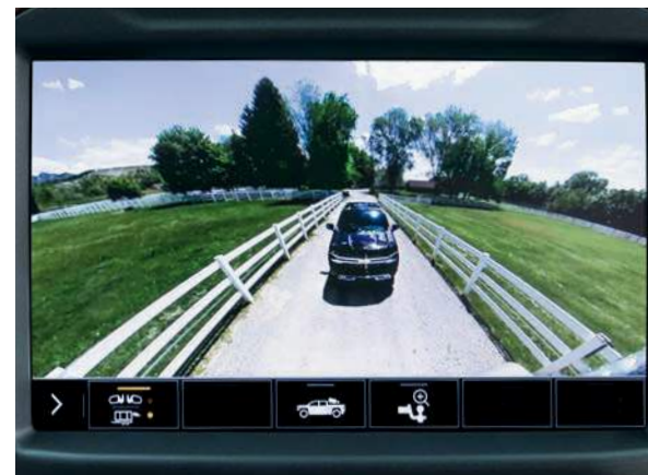
Rear Trailer View Uses an available accessory camera that can be installed to show vehicles or objects behind the trailer.
