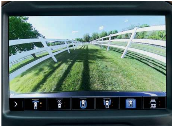
Front Camera View Displays front view with available guidelines to assist with parking and tight maneuvers.
