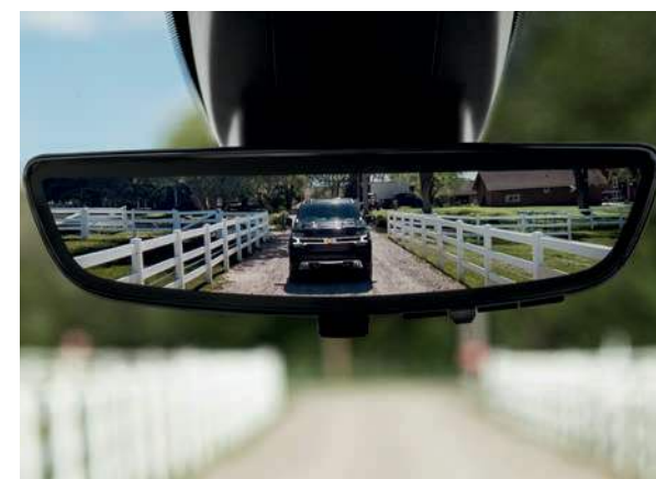
Rear Camera Mirror An available dual-function camera-based rearview mirror that provides a wider, less-obstructed field of view than a traditional rearview mirror.
