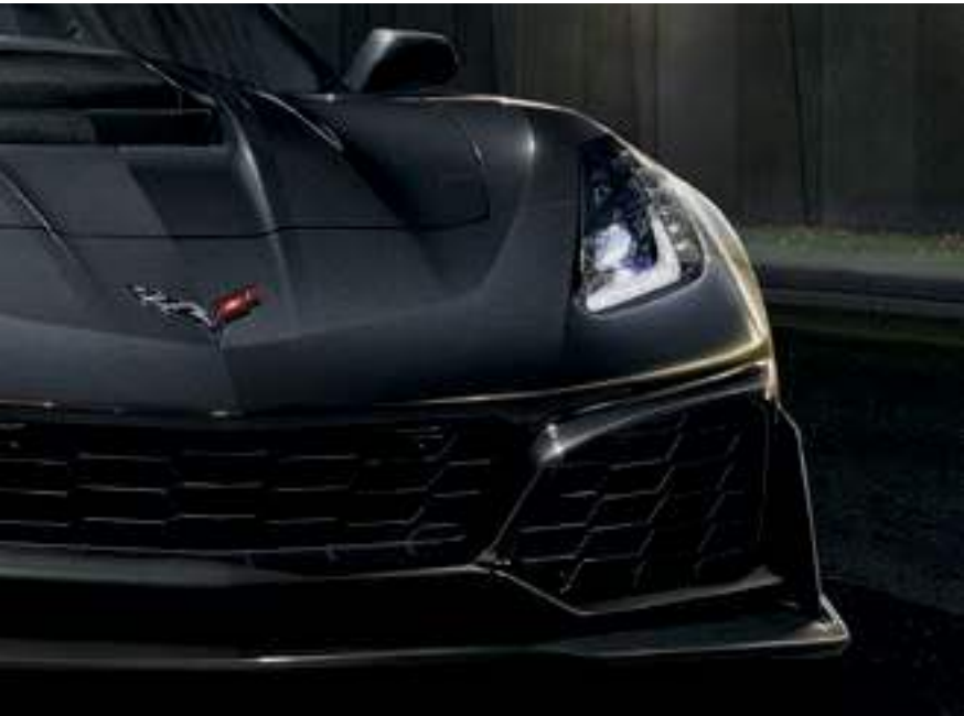
ADDITIONAL AIR INLETS ABOVE THE SPLITTER PROVIDE ENGINE COOLING AND MORE.
