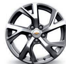
18" Machined-Face Aluminum with Painted Pockets (Standard on LT with 2.0L engine and Premier with 1.5L or 1.6L Diesel engine)
