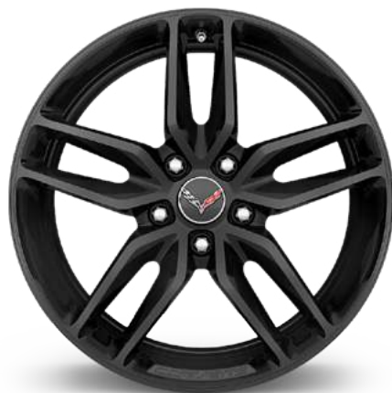
RPO Q7T 19" x 8.5" front and 20" x 10" rear Z51-style split 5-spoke Black aluminum
