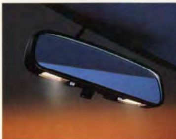
▲ An optional auxiliary light package includes an inside rearview mirror with built-in reading lamps.
