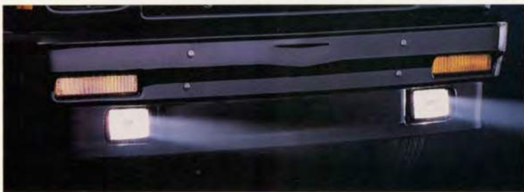
▲ Optional fog lamps can be ordered for standard air dam on 2WD models. Standard air dam on 4x4 models includes tow hooks.
