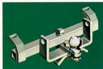
▲ Light-duty trailer hitch for hauling trailers up to 2000 lbs. with a maximum tongue load of 200 lbs. A 1-7/8"-diameter ball is included. (Dealer-installed accessory. See chart for part numbers.)
