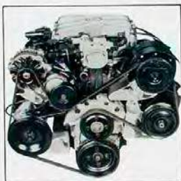
2.8 Liter V6 with Multi-Port Fuel Injection (standard on Camaro RS Coupe).
