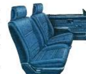
Optional CL Custom Cloth reclining bucket seats with adjustable lumbar support and vertical adjustment on driver's seat.
