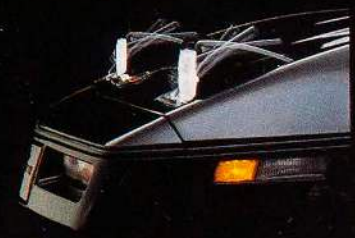
Powerful electric motors rotate the headlights.
