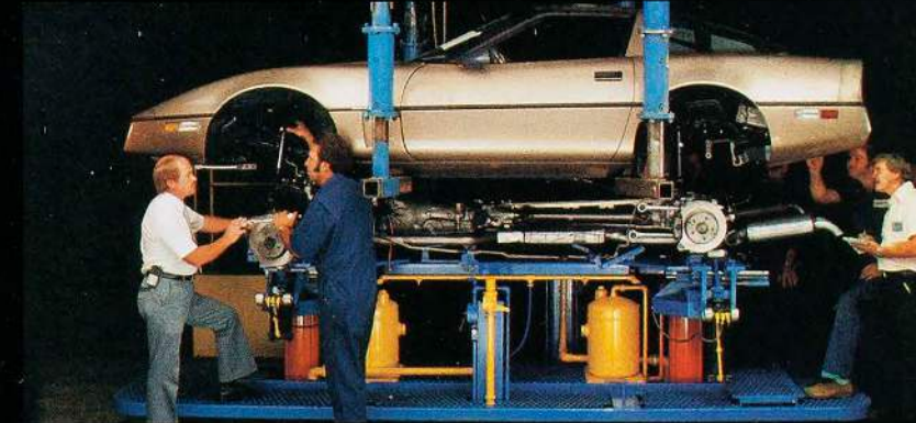
Specially built hydraulic towvever system "marries" chassis to body.
