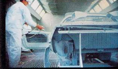
Clean-room environment is a key part of the paint process.
