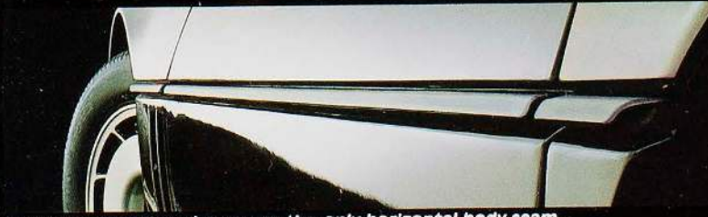
Protective molding also covers the only horizontal body seam.
