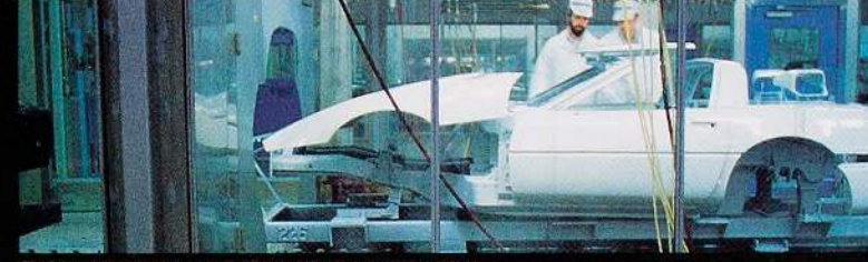
Between-coat inspection of Corvette paint.
