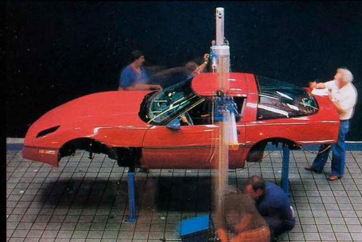
Point-check inspection to make sure body panel assembly meets design intent.
