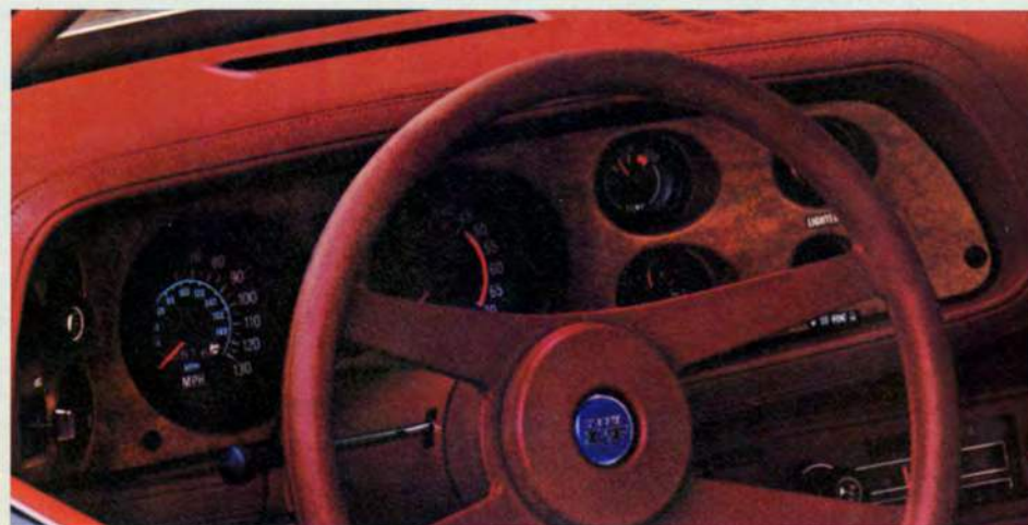
The Type LT instrument panel features a simulated leather instrument cluster facing, Special Instrumentation (tachometer, voltmeter, temperature gauge, electric clock), added instrument lighting, glovebox light and color-coordinated steering wheel with "Type LT" emblem.
