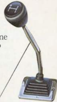
Standard 3-Speed transmission with floor-mounted shifter.
