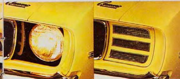
Concealed headlights, open. Concealed headlights, closed.
