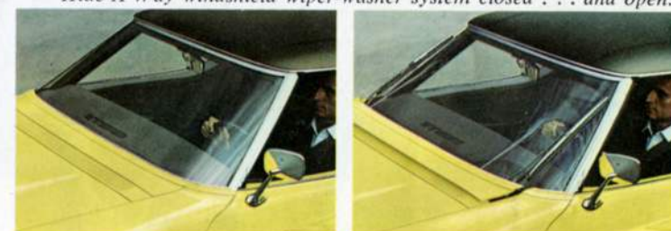
Hide-A-Way windshield wiper-washer system closed . . . and open.
