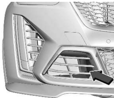
3. Front Brake Cooling Duct
