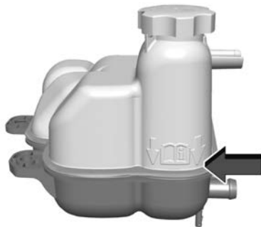
6.2L V8 Engine Coolant Surge Tank
