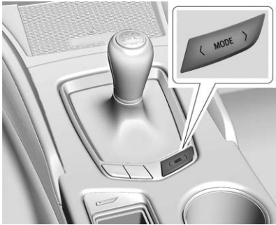
Driver Mode Control Switch for Manual Transmission
