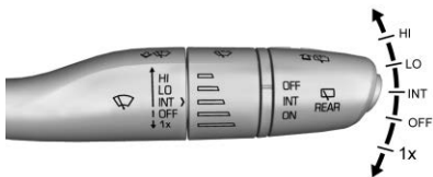
Windshield Wiper without Rainsense (INT Shown)
