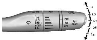
Windshield Wiper with Intermittent Wipers (INT Shown)
