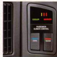
Dual automatic ComfortTemp climate control enables both driver and passenger to vary their own individual temperature levels by as much as four degrees.
