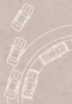
Standard anti-lock brakes help maintain steering control and prevent skidding when braking on most slippery surfaces.
