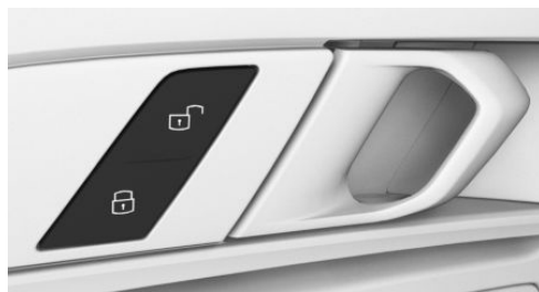
Buttons for the central locking system.
