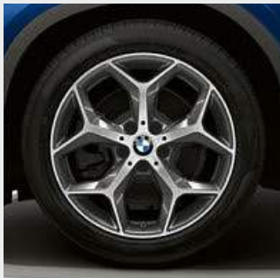
□ 18" light alloy Y-spoke style 569 wheels, Orbit Grey, 7.5J x 18 with 225/50 R18 tyres.
