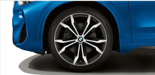
□ 20" M light alloy Double-spoke style 716 M wheels, 8J x 20 with 225/45 run-flat tyres.
