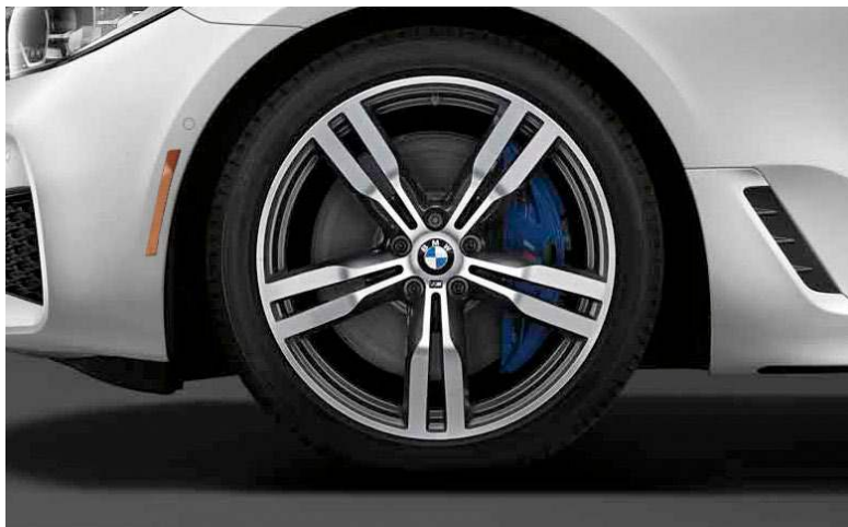
20" M Double-spoke wheels, style 648M, 20 x 8.5 front, 20 x 10.0 rear; and 245/40 front, 275/35 rear performance 1,2 run-flat 3 tires
