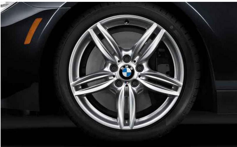
19" Double-spoke wheels, style 351M, 19 x 8.5 front, 19 x 9.0 rear; and 245/40 front, 275/35 rear performance 1,2 run-flat 3 tires 19 x 8.5; and 245/40 all-season 1 run-flat 3 tires
