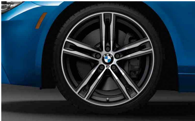
20" M Double-spoke wheels, style 703M, 20 x 8.5 front, 20 x 9.0 rear; and 245/35 front, 275/30 rear performance 1,2 run-flat 3 tires
