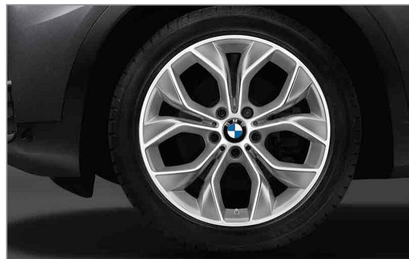
Y Spoke light alloy wheels (Style 608) 19 x 8.5 front and rear; and 245/45 front and rear run-flat all-season tires 2,3
