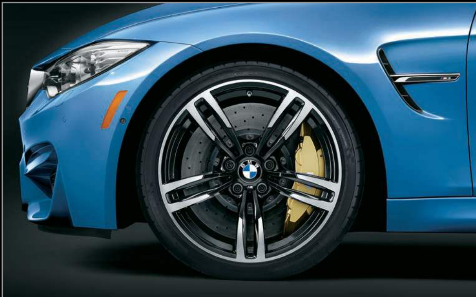
Black Double Spoke light alloy wheels (Style 437M) 19 x 9.0 front, 19 x 10 rear; and 255/35 front, 275/35 rear performance tires 1,2,3
