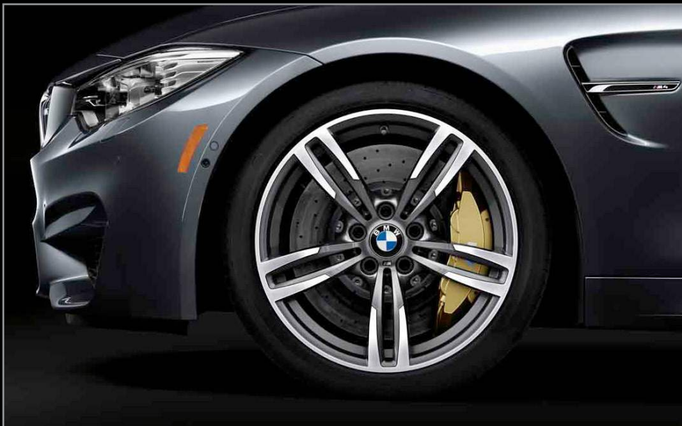
Double Spoke light alloy wheels (Style 437M), 19 x 9.0 front, 19 x 10 rear; and 255/35 front, 275/35 rear performance tires 1,2,3
