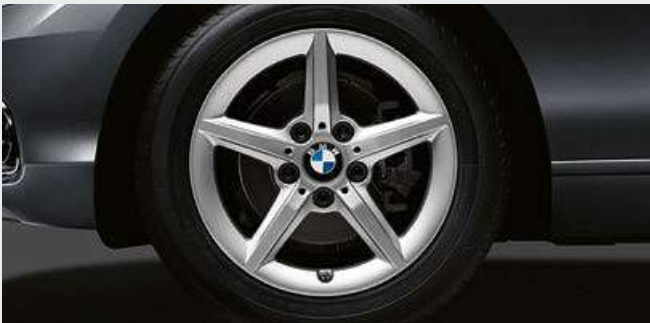
■ 16" light alloy Star-spoke style 654 wheels, 7J x 16 with 205/55 R16 tyres (Standard for SE models).
