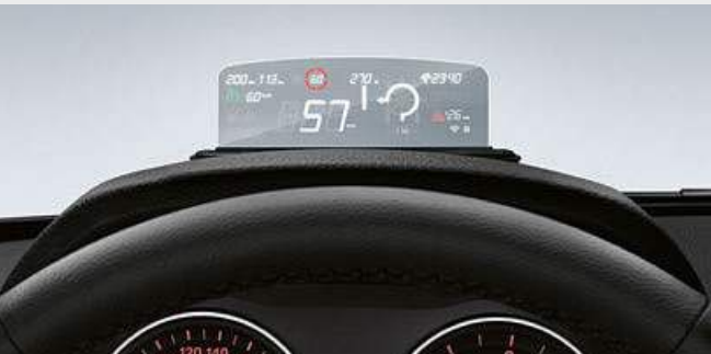
○ The BMW Head-Up Screen puts vehicle and navigation information into the driver's line of sight – in combination with a smartphone interface.
