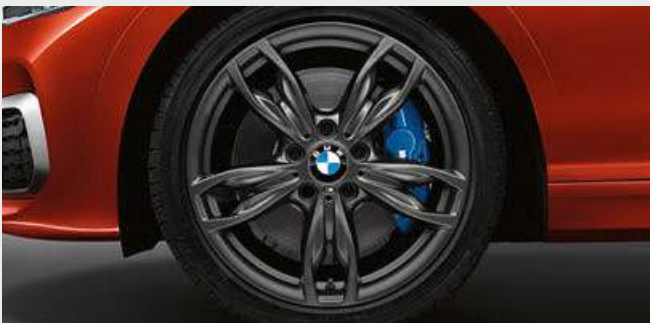
■ 18" M light alloy Double-spoke style 436 M wheels, Orbit Grey, front 7.5J x 18 with 225/40 R18, rear 8J x 18 with 245/35 R18 tyres (Standard for M140i Shadow Edition models).
