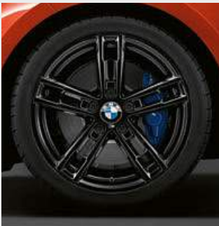
□ 18" M light alloy wheels Double-spoke style 719 M, Jet Black, front 7.5J x 18 with 225/40 R18, rear 8J x 18 with 245/35 R18 run-flat tyres.
