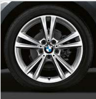
□ 18" light alloy Double-spoke style 385 wheels, front 7.5J x 18 with 225/40 R18, rear 8J x 18 with 245/35 R18 run-flat tyres.
