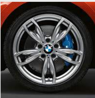
■ 18" M light alloy Double-spoke style 436 M wheels, Ferric Grey, front 7.5J x 18 with 225/40 R18, rear 8J x 18 with 245/35 R18 tyres (Standard for M140i models).
