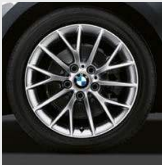
□ 17" light alloy Y-spoke style 380 wheels, 7J x 17 with 205/50 R17 run-flat tyres.
