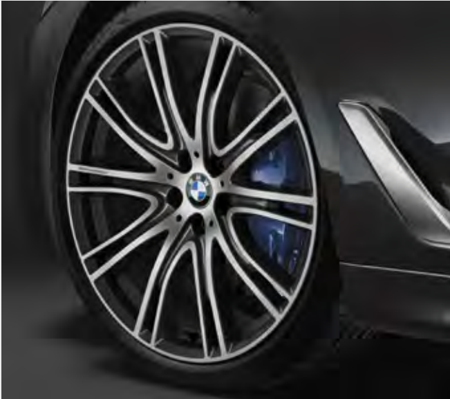
□ 20" BMW Individual light alloy V-spoke style 759 I wheels Bicolour, front 8J x 20 with 245/35 R20 tyres and rear 9J x 20 with 275/30 R20 tyres.
