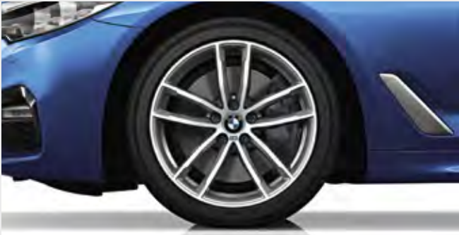
■ 18" M light alloy Double-spoke style 662 M wheels, front 8J x 18 with 245/45 R18 tyres, rear 9J x 18 with 275/35 R18 tyres. (Standard on 520d/520d xDrive M Sport models).
