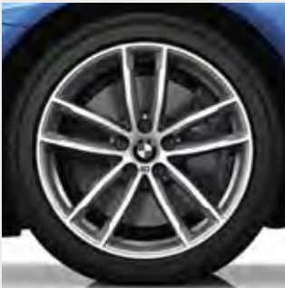
■ 18" M light alloy Double-spoke style 662 M wheels, front 8J x 18 with 245/45 R18 tyres, rear 9J x 18 with 275/35 R18 tyres. (Standard on 520d/520d xDrive M Sport models).
