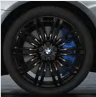
□ 19" M light alloy Double-spoke style 664 M wheels, Black, front 8J x 19 with 245/40 R19 tyres and rear 9J x 19 with 275/35 R19 tyres.
