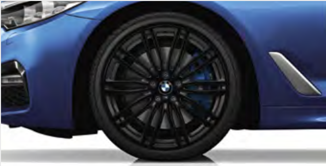
□ 19" M light alloy Double-spoke style 664 M wheels, Black, front 8J x 19 with 245/40 R19 tyres and rear 9J x 19 with 275/35 R19 tyres.
