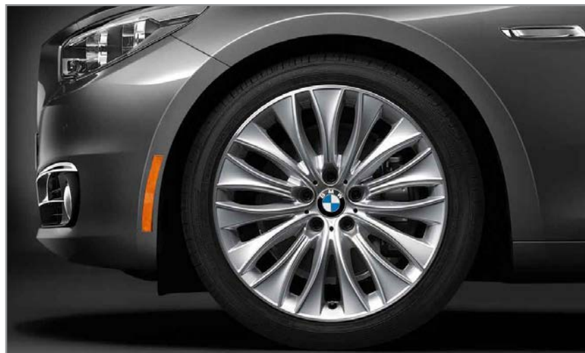
Multi-spoke light alloy wheels (Style 459) 20 x 8.5 front, 20 x 10.0 rear; and 245/40 front and rear 275/35 run-flat performance tires 2,3
