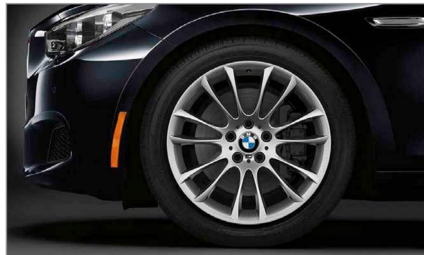
V Spoke light alloy wheels (Style 302M) 19 x 8.5 front and rear; and 245/45 front and rear run-flat all-season tires 1 19 x 8.5 front, 19 x 9.5 rear; and 245/40 front, 275/35 performance tires 1,2,3
