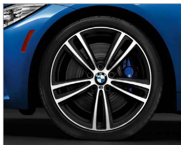
Double Spoke Orbit Gray light alloy wheels (Style 442M) 19 x 8.0 front and 19 x 8.5 rear; and 225/40 front and 255/35 rear performance tires 2,3
