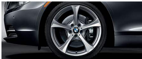
Star Spoke light alloy wheels (Style 276) , 18 x 8.0 front, 18 x 8.5 rear; and 225/40 front, 255/35 rear run-flat performance tires . 1 (Includes increased top-speed limiter).
