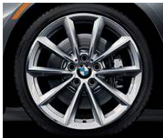
V Spoke light alloy wheels (Style 296) , 19 x 8.0 front, 19 x 9.0 rear; and 225/35 front, 255/30 rear run-flat performance tires . 1 (Includes increased top-speed limiter).
