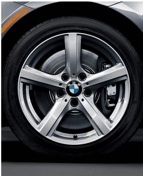
Star Spoke light alloy wheels (Style 290) , 17 x 8.0; and 225/45 run-flat performance tires . 1
