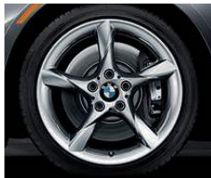
Star Spoke light alloy wheels (Style 295) , 18 x 8.0 front, 18 x 8.5 rear; and 225/40 front, 255/35 rear run-flat performance tires . 1 (Includes increased top-speed limiter).
