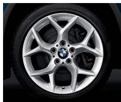
Y Spoke light alloy wheels (Style 322) , 18 x 8.0; and 225/45 run-flat 1 all-season tires. 2
