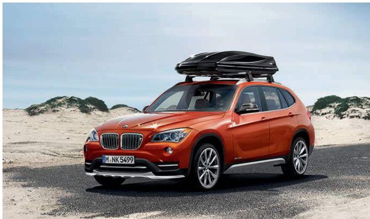
19-inch V Spoke Ferric Gray light alloy wheels (Style 324), BMW Replacement Performance Carbon-Fiber Mirror Caps, BMW Base Support System and BMW Roof Box 460 in Black.
