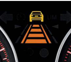
Active Cruise Control with Stop & Go 1 lets you preset desired speed and following distance. When it recognizes slower vehicles ahead, it reduces your speed to maintain the preset distance, and can even bring you to a complete stop if traffic calls for it. Active Cruise Control also includes the Active Driving Assistant features.
