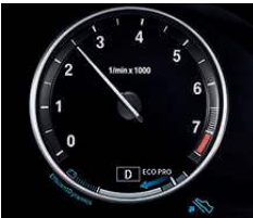
Driving Dynamics Control adjusts driving characteristics by pressing a button to select one of five settings. Choosing COMFORT, COMFORT+, SPORT, SPORT+ or ECO PRO mode adjusts the engine-throttle response, shift characteristics and power-steering assist. Another button disengages the traction control feature when driving on sand, gravel, or deep or packed snow.
