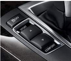
Driving Dynamics Control adjusts driving characteristics by pressing a button to select one of five settings. Choosing COMFORT, COMFORT+, SPORT, SPORT+ or ECO PRO mode adjusts the engine-throttle response, shift characteristics and power-steering assist. Another button disengages the traction control feature when driving on sand, gravel, or deep or packed snow.
