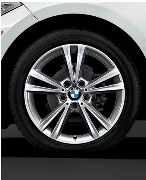
Double Spoke light alloy wheels (Style 385) with 18 x 7.5 and 225/40 run-flat¹ all-season tires².
