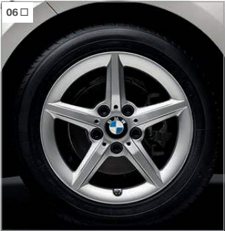
[ 05 ] The interior with standard seats in the optional cloth/leather combination 'Path' in Silver/Black is a classic example of driver-oriented BMW design. [ 06 ] 16" light alloy wheels Star-spoke style style 654, 7J x 16 with 205/55 R16 tyres.
