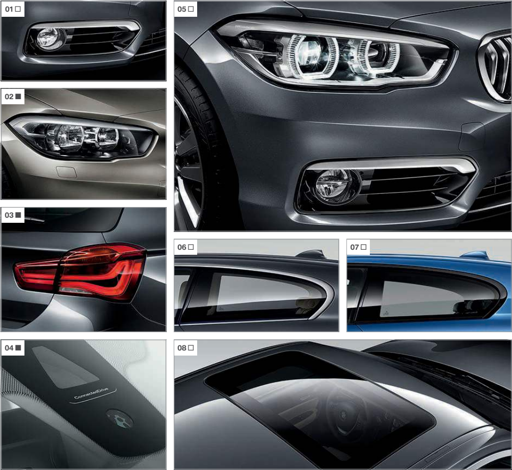
[ 01 ] The light generated by the LED fog lights 1 is very similar to daylight and enables the driver to see better and drive more safely in inclement weather. [ 02 ] The flat halogen double round headlights with LED daytime running lights accentuate the front's athletic look. [ 03 ] The two-part rear lights, including rear fog lights, are based on LED technology and are equipped with a dynamic brake light function. [ 04 ] The rain sensor including automatic headlight activation automatically switches on the windscreen wipers and the low-beam headlights. [ 05 ] Adaptive LED headlights including low-beam and high-beam headlights, LED turn indicators, LED fog lights and High-beam assistant. [ 06 ] The Chrome Line 2 Exterior with details in Chrome high-gloss gives the vehicle a particularly sophisticated look. [ 07 ] BMW Individual high-gloss Shadow Line 3 includes external equipment features in Black high-gloss. [ 08 ] The electric glass roof allows airflow to be regulated, creating a pleasant in-car climate. The integrated wind deflector guarantees a high level of acoustic comfort.
