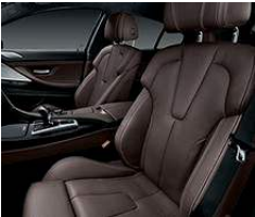
M Multi-contour seats for driver and front passenger. In addition to M seat adjustments, includes power upper backrest angle, backrest width and thigh support; comfort headrests with power height adjustment; lumbar support and memory function for driver and front passenger.
