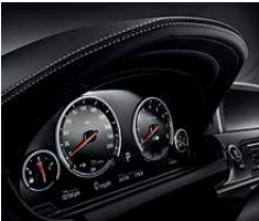
Instrument cluster features Black Panel Display with permanently illuminated white surrounds for speedometer and rev counter plus fuel level and oil temperature displays.
