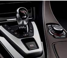
Gear shift lever for 7-speed M Double Clutch Transmission with Drivelogic includes M logo and illumination.
