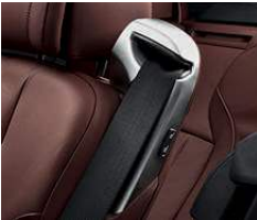
Integrated safety-belt system provides optimal protection and ergonomic comfort for the driver and front-passenger. The seat-integrated design also helps make entering and exiting the rear cabin easier.
