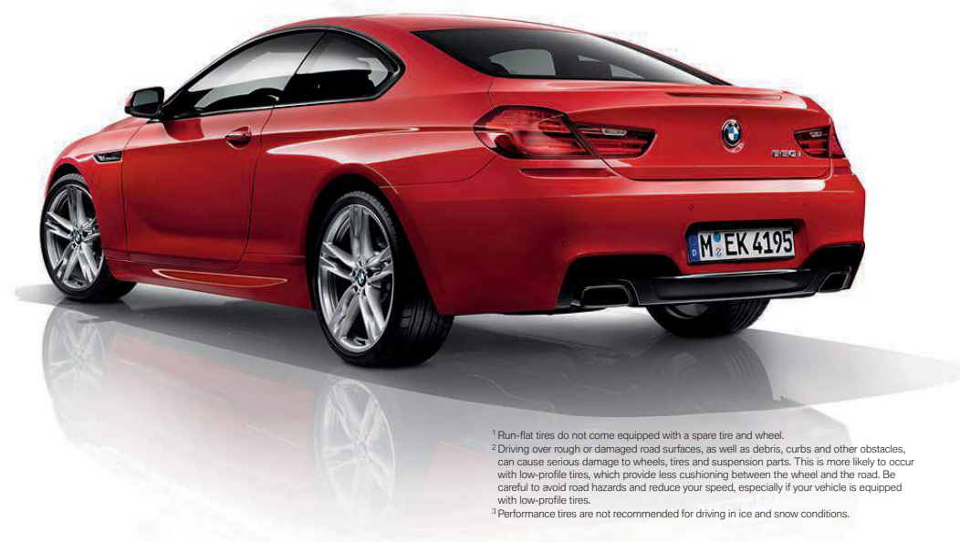
Double Spoke (Style 351M) light alloy wheels. With run-flat 1 performance tires 2,3 ; 19 x 8.5 front, 19 x 9.0 rear and 245/40 front, 275/35 rear tires. (Includes increased top-speed limiter.) With run-flat 1 all-season tires 2 : 19 x 8.5 wheels and 245/40 tires.
