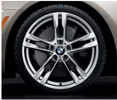
Double Spoke (Style 373M) 20 x 8.5 front, 20 x 9.0 rear light alloy wheels with 245/35 front and 275/30 rear run-flat 1 performance tires 2,3 (Includes increased top-speed limiter.)
