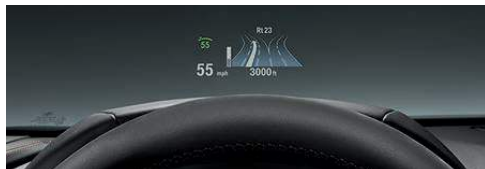
Full-color BMW Head-up Display projects important travel information, such as current speed, Navigation instructions, Speed Limit Info and Check Control data onto the windshield, directly in your line of sight.
