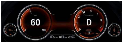
Dynamic Digital Instrument Cluster customizes the look of the instrument panel, based on your Driving Dynamics Control mode: COMFORT and COMFORT+, SPORT (shown) and SPORT+, or ECO PRO.
