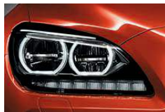
Adaptive LED Headlights for both high and low beams project an intense white light that simulates daylight for excellent visibility. LED foglights add a distinctive nighttime look.
