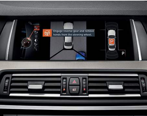
Parking Assistant makes parking a breeze by searching for suitable parking spots and then steering your vehicle into them. Simply press the "Park Assistant" button, then drive along potential parking spaces on the left or right side of the road, staying below 22 mph and no more than five feet away. Using ultrasonic sensors integrated into the side indicators, the system searches for and measures parking spaces. When a space at least four feet longer than your vehicle is spotted, it is shown on your Control Display. Shift into reverse and Park Assistant takes control of steering your vehicle into the selected space; you operate the accelerator and brake pedals. The acoustic and visual warnings of Park Distance Control (PDC) provide assistance.
