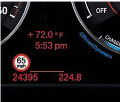
Speed Limit Info uses a camera installed close to the rear-view mirror to monitor posted speed-limit signs. Together with information supplied by the on-board Navigation system, it displays posted speed limits on the instrument cluster display and also in the Head-up Display.
