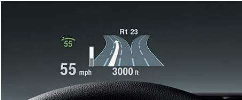
Head-up Display projects important travel information, such as current speed and Check Control data, on the windshield directly in your line of vision in full color. Also displayed are directional arrows from the Navigation system, Speed Limit Info and other driving warnings, if so equipped.
