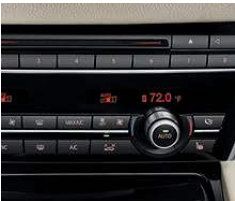
2-zone automatic climate control allows driver and front passenger to select individual temperatures and choice of fan speeds, as well as automatic or manual airflow and recirculation. The automatic recirculation control activates whenever certain air pollutants are detected. The system also offers a mist-up sensor, solar sensor and residual heat use.
