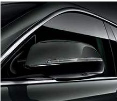
Heated, power-adjustable, folding exterior mirrors feature a body-color upper section, black bottom, and LED turn indicators. Passenger-side mirror tilts down when parking. Automatic dimming cuts headlight glare from any following vehicles.
