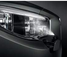
Retractable, high-intensity headlight washers help keep headlights clear of ice, mud, road salt and other coatings, for maximum road illumination and enhanced driving safety.
