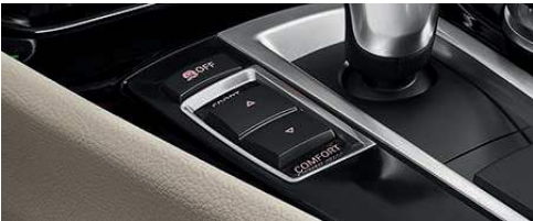
Driving Dynamics Control adjusts driving characteristics by pressing a button to select one of four settings. Choosing COMFORT, SPORT, SPORT+ or ECO PRO mode adjusts the engine-throttle response, shift characteristics and power-steering assist. Another button disengages the traction control feature when driving on sand, gravel, or deep or packed snow.
