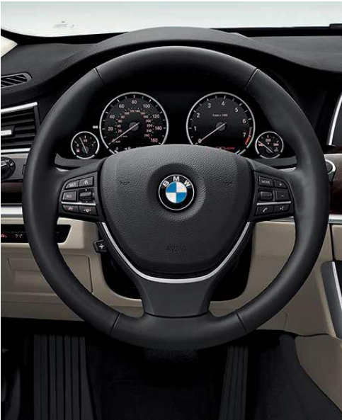
Three-spoke leather-wrapped multi-function steering wheel provides buttons on the left for cruise control functions, and buttons on the right for adjusting all audio-related functions, including a BMW-tested, Bluetooth® enabled mobile phone.
