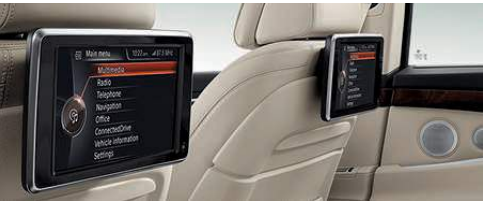
Rear-seat entertainment includes two tilt-adjustable, independently operated 9.2-inch color screens integrated into the back of the front seats. The system includes remote control and headphone jacks.
