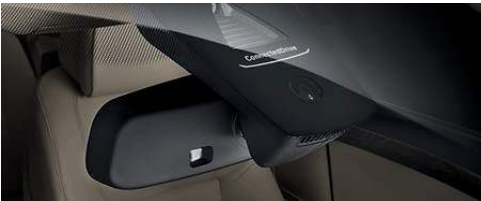
Rain sensor monitors the intensity of the rain and automatically regulates the windshield wiper interval. It also automatically turns on the low beams when needed.
