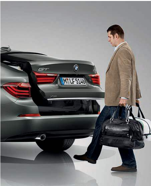
Comfort Access system offers convenient keyless access to the driver's door, front passenger door and tailgate when you carry the remote key in a pocket or purse, simply by touching the door handle. The hands-free trunk-lid opening function automatically unlocks and opens the trunk when you move your foot under the center of the rear bumper. Repeat the motion to close the trunk.
