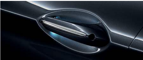
Soft-close function automatically closes all four doors shut for the last quarter inch.
