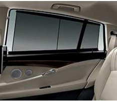
Sunblinds for the rear side windows can be electrically raised and lowered. They protect against intense sunlight while also providing effective privacy.
