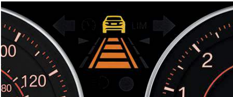
Active Cruise Control (ACC) with Stop & Go, including collision warning with brake activation lets you preset both desired speed and following distance. When ACC recognizes slower vehicles ahead, it reduces your speed to maintain the preset distance. Stop & Go can bring you to a complete stop if traffic calls for it. When you press the accelerator or resume ACC using the steering wheel, the system will resume your speed according to your settings. In critical situations, if necessary, collision warning with brake activation can intervene.
