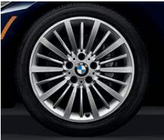
Multi-Spoke (Style 416) 18 x 8.0 light alloy wheels and 225/45 run-flat 1 all-season tires. 2
