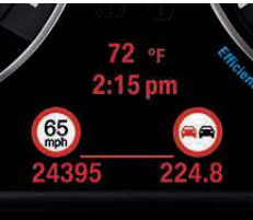
Speed Limit Info detects local speed limit signs and shows them in the Info Display and Head-up Display.
