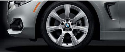
Star Spoke (Style 396) 18 x 8.0 light alloy wheels and 225/45 run-flat 1 all-season tires. 2
