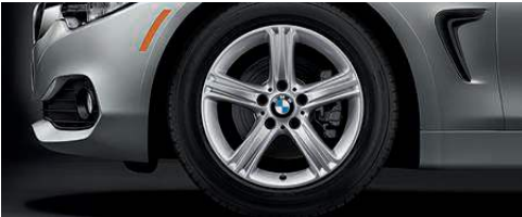
Star Spoke (Style 393) 17 x 7.5 light alloy wheels and 225/50 run-flat 1 all-season tires. 2
