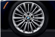
Multi Spoke (Style 416) 18 x 8.0 light alloy wheels and 225/45 run-flat 2 all-season tires 3 .
