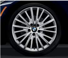
Multi-Spoke (Style 399) 19 x 8.0 front, 19 x 8.5 rear light alloy wheels and 225/40 front, 255/35 rear run-flat 1 performance tires . 2,3 (Includes increased top-speed limiter.)
