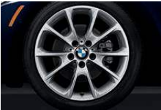
Double Spoke (Style 401) 1 19 x 8.0 front, 19 x 8.5 rear light alloy wheels and 225/40 front, 255/35 rear run-flat 2 performance tires 3,4 (Requires M Sport brakes; includes increased top-speed limiter.)
