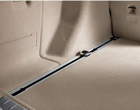
Aluminum rails with two adjustable latching eyes on the floor of the luggage compartment help secure bulky items during transport.
