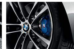
Optional M Sport brakes , featuring a fixed-calliper brake in dark blue with the "M" logo, enhance braking performance.
