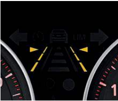
Lane Departure Warning 1 , a component of Active Driving Assistant, uses a camera to recognize when your vehicle is crossing over lane markings or is changing lanes without signaling, and warns you by sending a mild vibration through the steering wheel. The system can be turned on and off via a button by the steering wheel.
