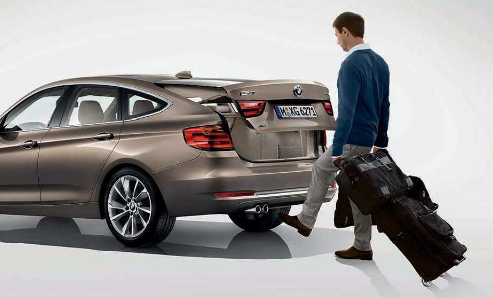
Comfort Access system offers convenient keyless access to your vehicle. Carrying the remote key in a pocket or purse allows you to unlock the doors by touching the door handle. The hands-free trunk-lid opening function automatically unlocks and opens the trunk when you stand behind the vehicle and move your foot under the center of the rear bumper.
