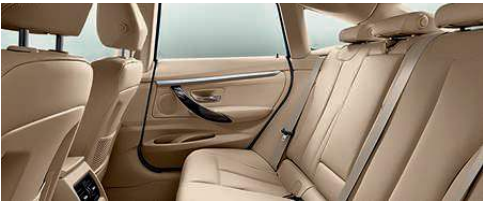
Tilt-adjustable rear seatbacks can be inclined in 15 stages.
