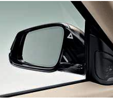
Active Blind Spot Detection warns if a vehicle is in your blind spot, or if a vehicle is approaching at high speed in the passing lane, by displaying a visual signal in the exterior mirror casing. The system also warns you by making the steering wheel vibrate should you then use the turn-signal indicator before executing a lane change.
