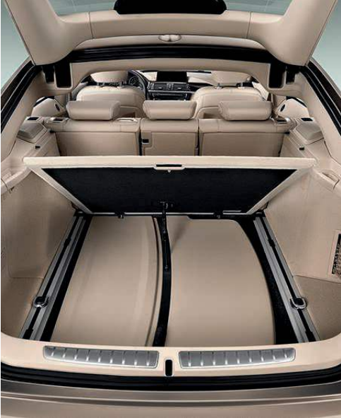
Removable two-part cargo cover opens automatically when the tailgate is lifted. Once removed, it can be easily stored under the floor of the luggage compartment (as shown above).
