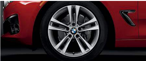
Double Spoke (Style 397) 18 x 8.0 light alloy wheels and 225/45 run-flat 1 performance tires . 2,3 (includes increased top-speed limiter) or run-flat 1 all-season tires . 2
