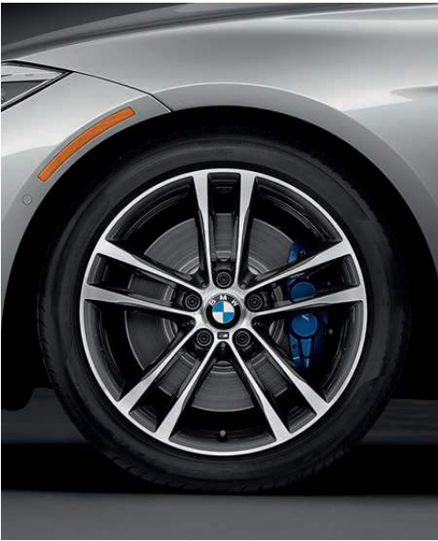
Double Spoke (Style 598M) 19 x 8.0 front, 19 x 9.0 rear light alloy wheels and 225/45 front, 255/40 rear summer tires . 2,3 (Includes increased top-speed limiter.)
