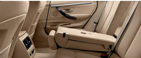
Rear passenger compartment includes 40/20/40 split-folding seat backrests for flexible passenger/cargo configurations.
