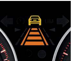
Active Cruise Control (ACC) with Stop & Go. 2 This system lets you pre-set both desired speed and following distance. When ACC recognizes slower vehicles ahead, it reduces your speed to maintain the preset distance. Stop & Go can bring you to a complete stop if traffic calls for it. Press the accelerator or use the steering wheel control to resume your speed according to your settings.
