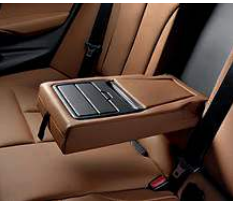
Rear center armrest includes two cupholders integrated into the front of the armrest. When not in use, they can be stored out of sight by sliding them back into the armrest. The armrest swings up to create a third rear passenger seat.
