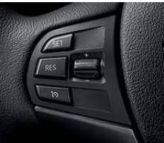
Dynamic Cruise Control 2 lets you set and keep to a chosen speed above 20 mph, including automatic application of the brakes when driving downhill. It is activated and regulated via controls positioned on the left side of the steering wheel, and deactivated by applying the brakes or switching off the feature.
