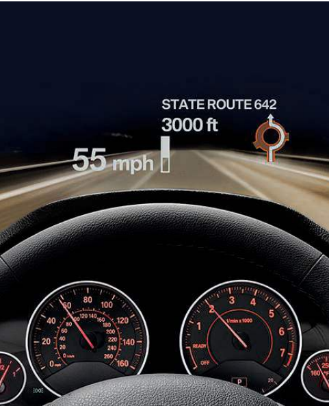
Head-up Display projects important travel information, such as vehicle speed and Check Control warnings, onto the windshield directly in your field of vision. Data is shown in full color, making information even more precise and easier to process. Additional information, including Navigation directional arrows and instructions, can also be displayed.
