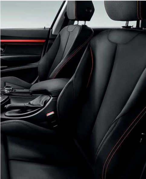
10-way power front sport seats make the driving experience more enjoyable with adjustments for fore/aft, seat height, backrest angle and seat angle. Side bolsters can be power-adjusted to comfortably fit your back while helping to hold you firmly in place during cornering. Includes two-way headrests with Active Head Restraints feature. Heated front seats are a welcome feature in cooler weather. By pressing the icon button, the seating surfaces – seat bottom, backrest and sides – are heated to your choice of three settings. Heated rear seats offer multiple settings to warm the seat bottoms and backrests of the left and right seats.
