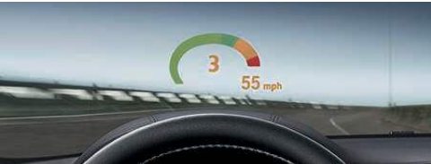
BMW Head-Up Display projects important travel information, such as current speed and Check Control data, directly into your line of vision in full color. It also, among other functions, shows the dynamic rev band, gear-selection indicator and the Shift Light function via an M-specific color display. Directional arrows from the Navigation system can also be displayed.
