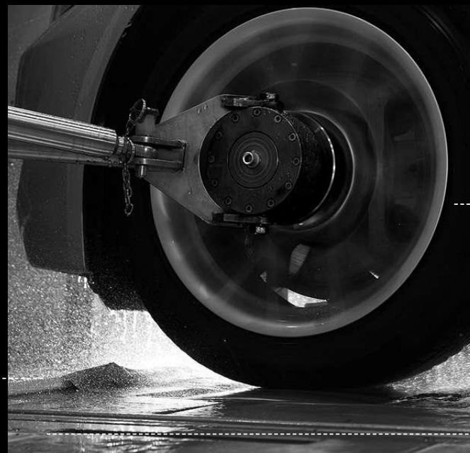
Secured: during the evaluation, the vehicle is anchored to the test bed (left). Solarium: high-power radiant lamps in the ceiling simulate strong sunshine.
