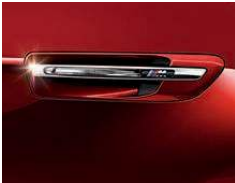
M gill elements with side indicator and M logo in the sidewall (BMW X6 M design).
