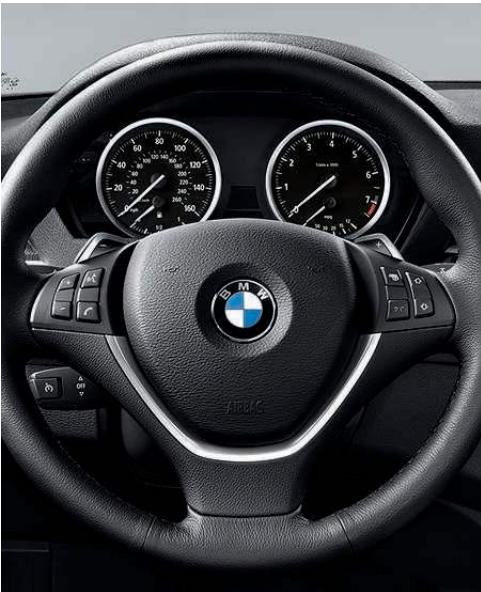
Three-spoke leather-wrapped multi-function sport steering wheel , featuring power tilt/telescoping adjustments, lets you keep both hands on the steering wheel while adjusting both the audio and a BMW-approved, Bluetooth® enabled mobile phone.
