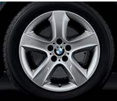
Star Spoke (Style 212) 19 x 9.0 light alloy wheels with 255/50 run-flat 1 all-season tires.
