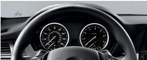
Instrument cluster features four analog displays for speed, rpm, fuel level and fuel consumption, as well as the Info Display that shows, for example, the exterior temperature and the functions of the on-board computer.
