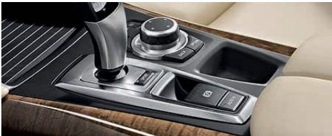
Electromechanical parking brake with Automatic Hold keeps the vehicle stationary whenever the vehicle comes to a stop, then releases the brake when the driver steps on the accelerator pedal. Sport button allows selection of a firmer suspension setting when equipped with Adaptive Drive.
