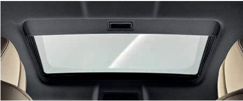
Two-way power glass moonroof with remote, expanded one-touch operation, slides back or tilts up to let in as much fresh air and sky as you like, while a wind deflector helps keep the wind out. Includes a sliding interior sunshade.
