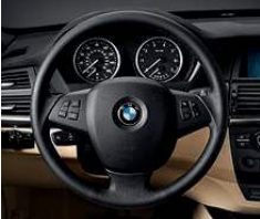
Three-spoke leather-wrapped multi-function steering wheel provides buttons on the left for operating the cruise control functions and buttons on the right for adjusting all audio-related functions, including a BMW-approved, Bluetooth® enabled mobile phone, if so equipped.
