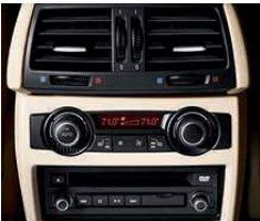
4-zone automatic air conditioning builds on the 2-zone system with air vents in the B-pillar and at the rear of the center console, to ensure virtually draftless ventilation for rear-seat passengers. Additionally, the temperature in both left and right rear cabin can be tailored via two control dials with displays.
