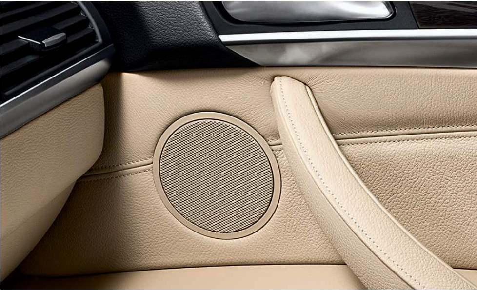
Premium high-fidelity system is a 16-speaker, multi-channel system that outputs reproduction of the surround information contained in the stereo signal in a nine-channel format (seven mid- and high-range channels and two central bass channels) as well as 5.1 surround-sound from a DVD source. Includes a 600-watt digital amplifier with nine channels. The system compensates for driving noise in smooth steps with speed-dependent equalizing. All speakers are fitted with very strong, yet compact neodymium drives.
