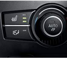
Heated front seats are a welcome feature in cooler weather. With the touch of a button, driver and front passenger can individually select from three heat settings.
