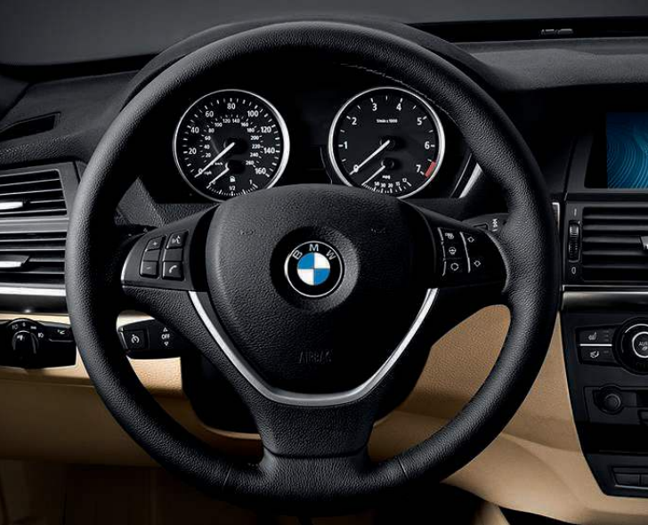
Three-spoke leather-wrapped multi-function sport steering wheel , featuring power tilt/telescoping adjustments, lets you keep both hands on the steering wheel while adjusting both the audio and a BMW-approved, Bluetooth enabled mobile phone, if so equipped. The right-hand buttons are used to operate all cruise control functions, while those on the left serve the audio functions, such as the radio, telephone and Voice command, if so equipped.
