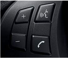
Voice command lets you verbally control numerous Navigation system functions and dial phone numbers hands-free. The Voice command button must be pressed before each use, so conversations won't accidentally activate the phone or other systems. (Voice command is part of the Navigation system.)
