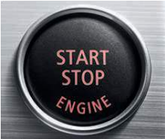
Engine Start/Stop button and remote key control the engine. First, insert the remote key into the starter switch slot. After the electronic identification system confirms that it is the correct remote key, you can start (or later, turn off) the engine by pressing the Start/Stop button. (Foot must be on brake in order to start.)
