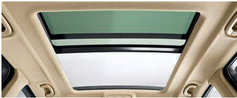
Panoramic moonroof is designed with generous dimensions to offer a stunning view, day or night. Easy-to-use features include a power slide and lift control, a comfort opening/closing function, a speed-sensitive wind deflector, and a power sunshade to shield passengers from excessive glare and heat. Both glass panels tilt up electronically at the touch of a button; the front panel also features a sliding function.
