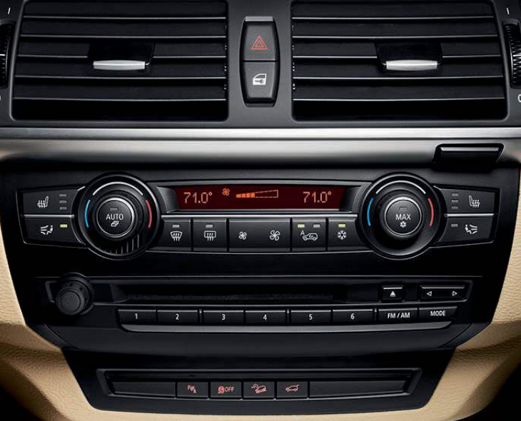
2-zone automatic climate control allows driver and front passenger to select individual temperatures and choice of fan speeds, as well as choose automatic or manual airflow and recirculation. The automatic recirculation control activates whenever certain air pollutants are detected. The system also offers a mist-up sensor, solar sensor and residual heat use.
