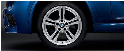
Double Spoke (Style 355M) 18 x 8.0 front, 18 x 9.0 rear light alloy wheels with 225/45 front, 255/40 rear run-flat¹ performance tires.²,³
