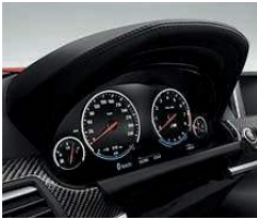
Extended instrument cluster features Black Panel Display with permanently illuminated white surrounds for speedometer and rev counter plus fuel level and oil temperature displays.
