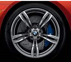
Double Spoke (Style 343M) 20 x 9.0 front, 20 x 10.0 rear forged light alloy wheels with 265/35 front, 295/30 rear run-flat 1 performance tires. 2
