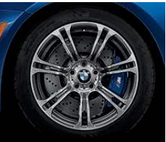
Star Spoke (Style 344M) 19 x 9.5 front, 19 x 10.5 rear forged light alloy wheels with 265/40 front, 295/35 rear run-flat 1 performance tires. 2
