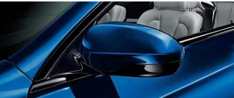
M wing mirrors in body color are heated and electrically adjustable. The mirror base and lower part of the mirror case are painted in high-gloss black.
