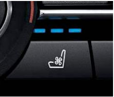
Active Ventilated seats gently blow warm or cool air through the micro-perforations in the leather to keep seat occupants comfortably dry in hot weather and warm in colder weather.
