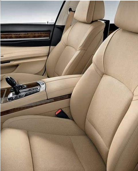
20-way Multi-contour seats conform to your body to provide optimum support and exceptional comfort over long distances. In addition to horizontal, vertical and angled adjustments, seats include an articulated upper backrest, adjustable backrest width, adjustable thigh and adjustable side support, Comfort headrest (two-way power, two-way manual "relax headrest"), and four-way power-adjustable lumbar support. Both driver's and front-passenger's seats also include Active Head Restraints and memory function.
