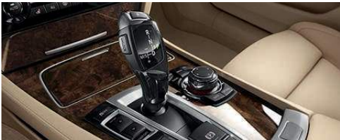
8-speed STEPTRONIC automatic transmission with Adaptive Transmission Control (ATC) provides extremely fast synchronized shifting in either the Sport or Manual shift mode. By increasing the number of gears to eight, the transmission provides a more efficient shifting sequence and improved fuel economy.
