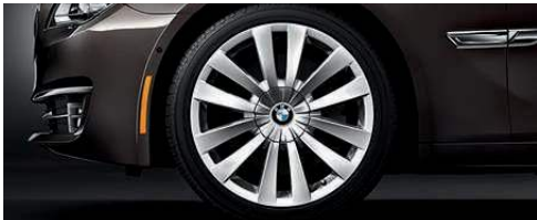
Double Spoke (Style 253) 20 x 8.5 front, 20 x 10.0 rear light alloy wheels with 245/40 front, 275/35 rear run-flat¹ performance tires.²,³
