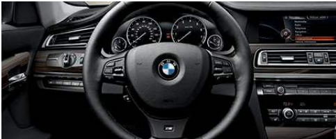
Three-spoke leather-wrapped multi-function M sport steering wheel includes a thick, textured rim and thumb indents designed for performance driving. Racecar-inspired steering wheel-mounted paddle shifters let you upshift and downshift, while multi-function buttons allow you to adjust various comfort features while keeping both hands on the wheel.
