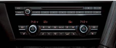
2-zone automatic climate control allows driver and front passenger to select individual temperatures and choice of fan speeds, as well as choose automatic or manual airflow and recirculation. The automatic recirculation control activates whenever certain air pollutants are detected. The system also offers a mist-up sensor, solar sensor and residual heat use.
