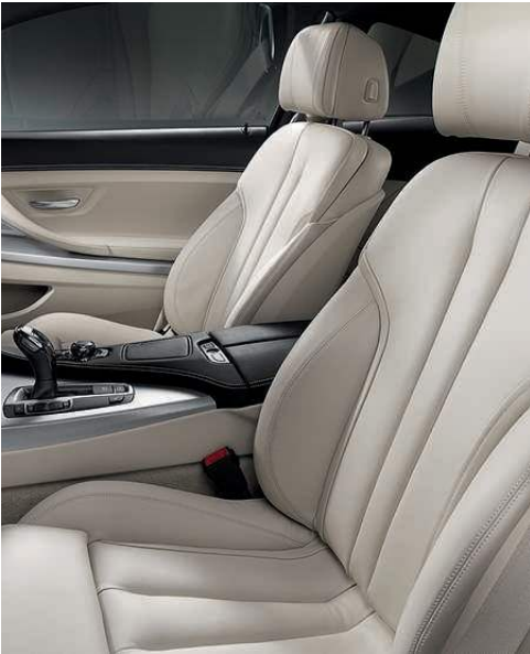
20-way power Multi-contour front seats conform to your body to provide optimum support and exceptional comfort over long distances. In addition to horizontal, vertical and angled adjustments, Multi-contour seats include an articulated upper backrest, comfort headrest (two-way power, two-way manual "relax headrest"), and four-way power-adjustable lumbar support. Both driver's and front-passenger's seats include memory function. Active front seats (not shown) imperceptibly raise and lower the left and right halves of the seating surface. This movement keeps the spine in motion, exercising various support muscles to help reduce fatigue on longer trips. Ventilated front seats (not shown) gently blow warm or cool air through the micro-perforations in the leather to keep driver and front passenger comfortably dry in hot weather, and warm in colder weather.
