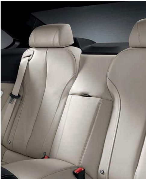
Rear seating consists of two individual leather-covered seats. Both include an ergonomic belt system with integrated belt catches, two three-point safety belts and headrests. A LATCH child-seat fastening system is also included.
