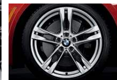
Double Spoke (Style 373M) 20 x 8.5 front, 20 x 9.0 rear light alloy wheels with 245/35 front and 275/30 rear run-flat performance tires . 1
