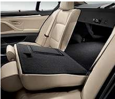
Rear seat backrests can be folded individually in a 60/40 split to optimize the number of passengers and amount of cargo. Ski bag accommodates up to four pairs of skis or other long objects for practical transport inside the vehicle. The bag protects transported items while simultaneously protecting the vehicle interior from damage.
