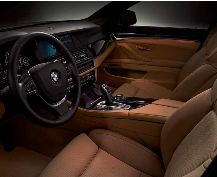
Ambiance lighting adds the drama of a warm reddish light that runs from front to rear beneath the inner door ledge. Interior lighting also includes soft white rear reading and footwell lights, illumination of the front center armrest storage compartment, indirectly lit door pockets, exit lights, and proximity illumination in the outside door handles.
