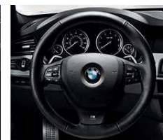
Three-spoke, leather-wrapped multi-function M sport steering wheel includes a thick, textured rim and thumb indents that are designed for performance driving.
