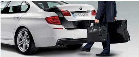
Comfort access system offers convenient keyless access to your vehicle when you carry the remote key in a pocket or purse. The hands-free trunk-lid opening function automatically unlocks and opens the trunk when you stand behind the vehicle and move your foot under the center of the rear bumper. You can also unlock the doors merely by touching the door handle. Automatic soft-close feature uses small electric motors to gently pull all four doors shut the last few inches.
