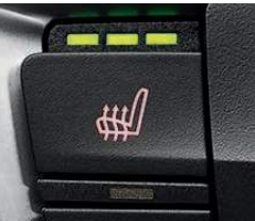
Heated front seats are a welcome feature in cooler weather. By pressing the icon button, the seating surfaces – seat bottom, backrest and sides – are heated to your choice of three settings. Heated rear seats offer multiple settings to warm the seat bottoms and backrests of the left and right seats.
