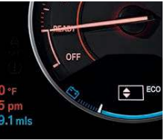
Auto Start-Stop function – and on the BMW ActiveHybrid 3, the Hybrid Start-Stop function – switches off the engine automatically during brief stops, such as at red lights, to reduce fuel consumption. A symbol displayed in the rev counter indicates that the function is active.
