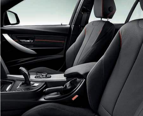
Front sport seats offer ten-way power adjustment including two-way manual adjustment of headrests. The driver's seat provides individual adjustments for seat height and backrest, fore and aft position and seat angle.
