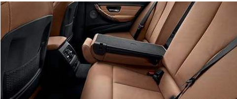
Rear fold-down seats allow flexible combinations of passengers and cargo. Use the folding 40-20-40 seats with through-loading feature for transporting skis or other long items.
