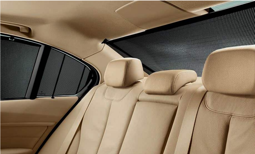
Power sunshade for the rear window can be raised and lowered at the press of a button. Together with manual sunshades for the rear side windows, this feature maintains occupant privacy, helps eliminate glare, and helps lower the cabin temperature by reflecting intense sunlight. (European model shown.)
