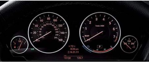
Instrument panel features a red backlit speedometer and tachometer. Centered between the two easy-to-read analog instruments is the on-board computer with liquid crystal display providing additional important driving information. Extended instrument cluster , included with the Navigation system, has a high-resolution Info Display showing functions for the Check Control as well as Navigation system prompts and operational feedback. With the ECO PRO mode activated, EfficientDynamics information is displayed in the rev counter.
