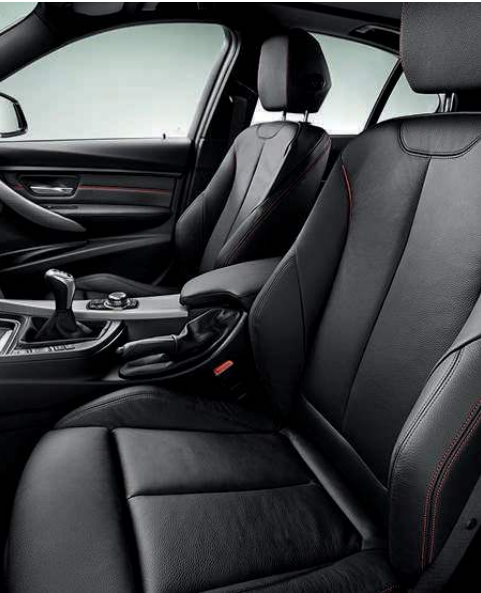
12-way power front sport seats make the driving experience more enjoyable with adjustments for fore/aft, seat height, backrest angle, seat angle and thigh support. Side bolsters can be power-adjusted to comfortably fit your back while helping to hold you firmly in place during cornering. Includes two-way headrests with Active Head Restraints feature.
