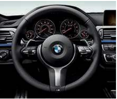
Three-spoke, leather-wrapped multi-function M sport steering wheel includes a thick, textured rim and thumb indents that are designed for performance driving. Multi-function buttons let you adjust various comfort features while keeping both hands on the wheel.
