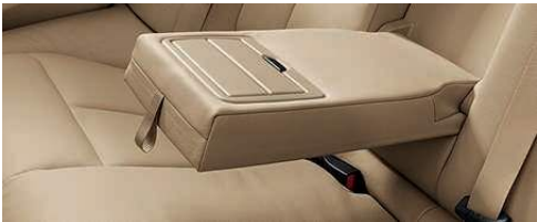
Rear center armrest includes two cupholders integrated into the front of the armrest. When not in use, they can be stored out of sight by sliding them back into the armrest. The armrest swings up to create a third rear passenger seat.
