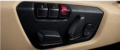
Power seat adjustment for driver and front passenger customizes seat height, seat and backrest angle, and fore/aft position. Includes a two-driver memory function for driver's seat and power-folding exterior mirrors.
