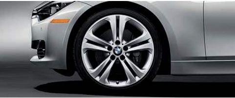
Double Spoke (Style 401) light alloy wheels and run-flat 1 performance tires. 2 In front: 19 x 8.0 wheels and 225/40 tires; in back: 19 x 8.5 wheels and 255/35 tires.
