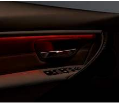
Lighting package features vicinity lighting in the outside door handles. Inside, includes Ambiance lighting front and rear, front footwell lights, vanity mirror lighting in front sunshades, and LED lighting in the front door handles, reading lights front and rear, and in the trunk.
