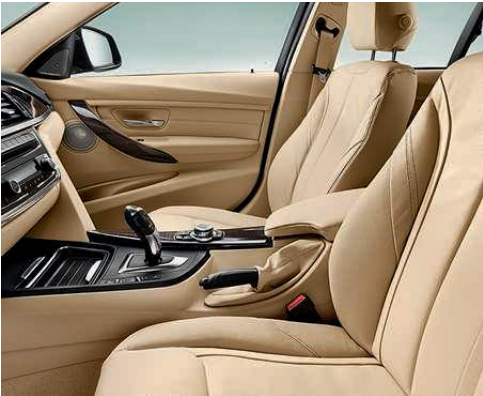
Power front seats offer eight-way power adjustment including two-way manual headrests. The driver's seat provides individual adjustments for seat height and backrest, fore and aft position and seat angle.
