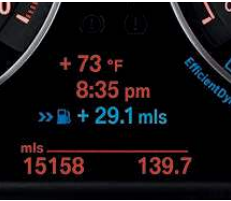
On-board computer provides data on exterior temperature, average speed, average and current fuel consumption, and range. With the ECO PRO mode activated, the current bonus range is also displayed.
