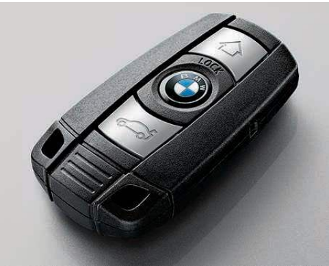
Comfort Access system offers convenient keyless access to your car. Simply carrying the remote key in a pocket or purse allows you to lock or unlock the doors by touching the door handle. You can also turn the engine on or off by pressing the Start/Stop button without inserting the remote key. (Foot must be on the brake; with manual transmission, clutch must also be depressed in order to start.)
