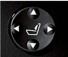
Lumbar support for front seats adds four-way power-adjustable comfort for the lower back. Lumbar support can be adjusted up/down and in/out for an ergonomically perfect seatback position and support of the back muscles.
