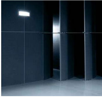
To the rear of the test track, tall hemispherical partitions guide the airflow back in the opposite direction.
