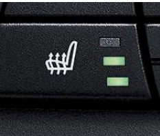
Heated front seats are a welcome feature for driver and front passenger in cooler weather. By pressing the icon button, seat surface and backrest are heated and quickly radiate comfortable warmth in your choice of three settings.
