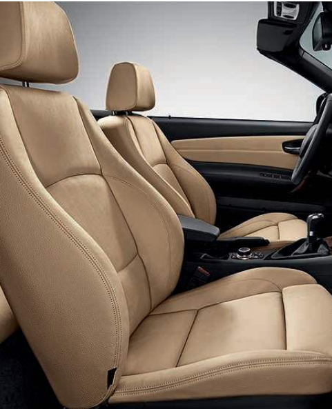
Eight-way adjustable front sport seats , included in the 135is or M Sport Package, make the driving experience more enjoyable. Side bolsters can be power-adjusted to fit your back comfortably while helping to hold you firmly in place during tight cornering. Includes two-way headrests and thigh support for added support.
