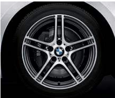
18-inch Double Spoke (Style 313M) light alloy wheels with run-flat 1 performance tires. 2 In front: 18 x 8.0 wheels with 225/40 tires; in back: 18 x 8.5 wheels with 255/35 tires.
