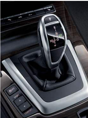
Driving Dynamics Control allows you to tailor the Z4's performance by selecting COMFORT, SPORT or SPORT+ driving modes at the touch of a switch. This changes throttle response, steering assist, suspension damping (with Adaptive M Suspension) and automatic transmission shifting (if so equipped). Additionally, you can deactivate Dynamic Stability Control (DSC) and switch to Dynamic Traction Control (DTC), which allows wheelslip within defined limits when driving in deep snow, or for a sportier driving style. Adaptive M Suspension lowers the chassis by 0.4 inches and electronically adjusts the dampers from sportingly tight to relaxed and comfortable, for greater agility and precise response.
