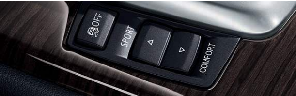
Driving Dynamics Control allows you to tailor the Z4's performance by selecting COMFORT, SPORT or SPORT+ driving modes at the touch of a switch. This changes throttle response, steering assist, suspension damping (with Adaptive M Suspension) and automatic transmission shifting (if so equipped). Additionally, you can deactivate Dynamic Stability Control (DSC) and switch to Dynamic Traction Control (DTC), which allows wheelslip within defined limits when driving in deep snow, or for a sportier driving style. Adaptive M Suspension lowers the chassis by 0.4 inches and electronically adjusts the dampers from sportingly tight to relaxed and comfortable, for greater agility and precise response.
